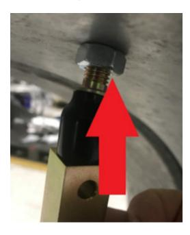
2. Loosen outer Locknut
