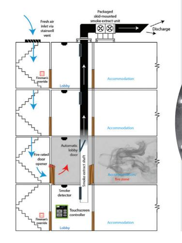
• The system provides a dedicated mechanical extraction point on each floor. • In the event of a fire, where the system is activated on any one floor; an evacuating occupant will exit from the office to the lobby and then into the
