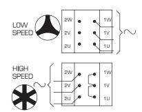
WARNING CONTROL GEAR FOR THIS POLE MOTOR
